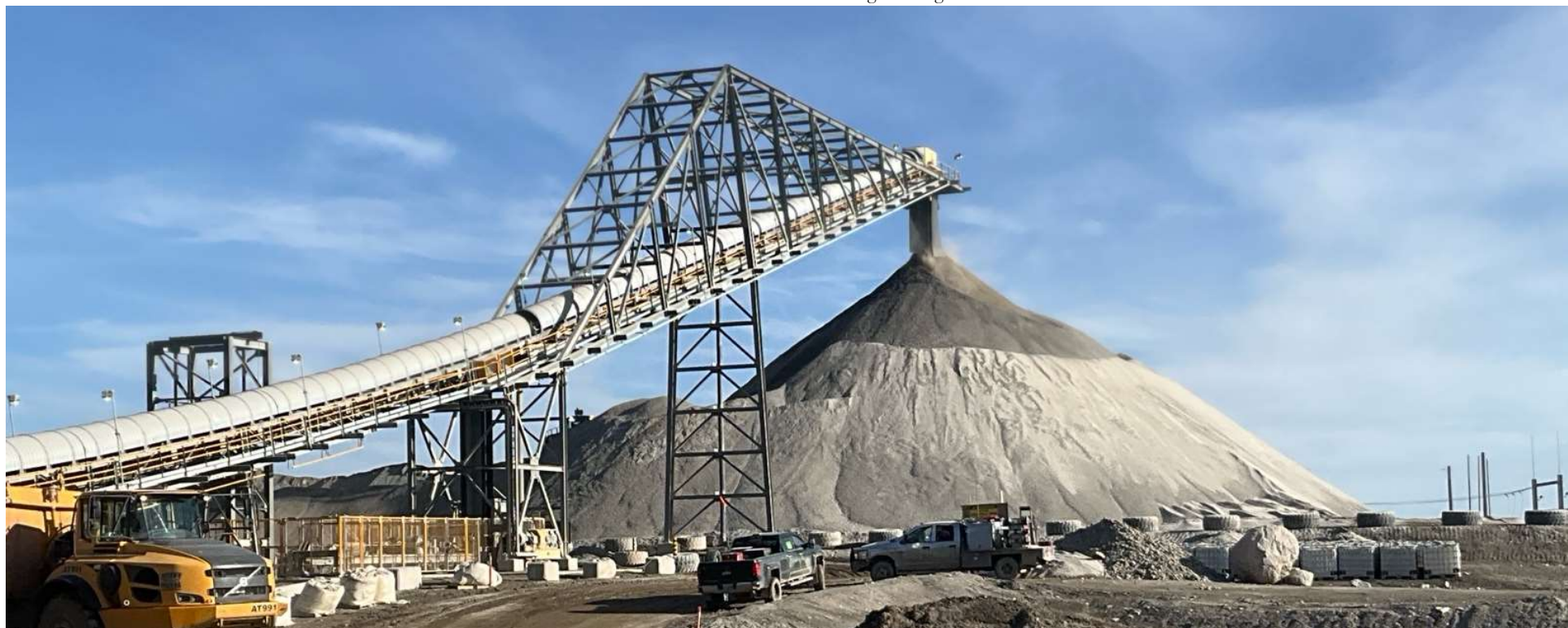
Photo 113701-2. Overview of the drop point to the stockpile at the terminus of the crusher conveyor circuit at the Plant Site.
