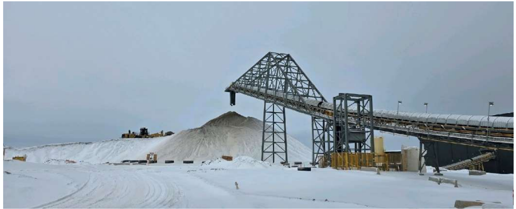
Photo 113115-1. High grade ore stockpile being worked and fed to plant site at the terminus of the crusher circuit.
