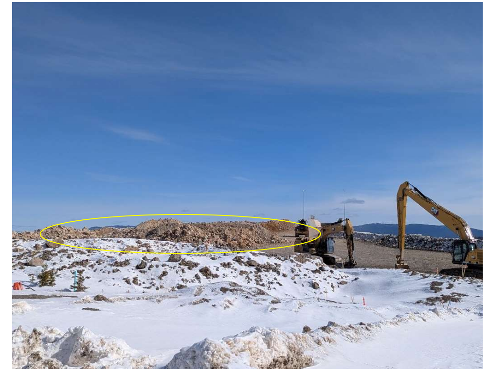
Photo 113344-3. High-grade ore stockpiled on the ROM pad being fed into the conveyor/crusher system.
