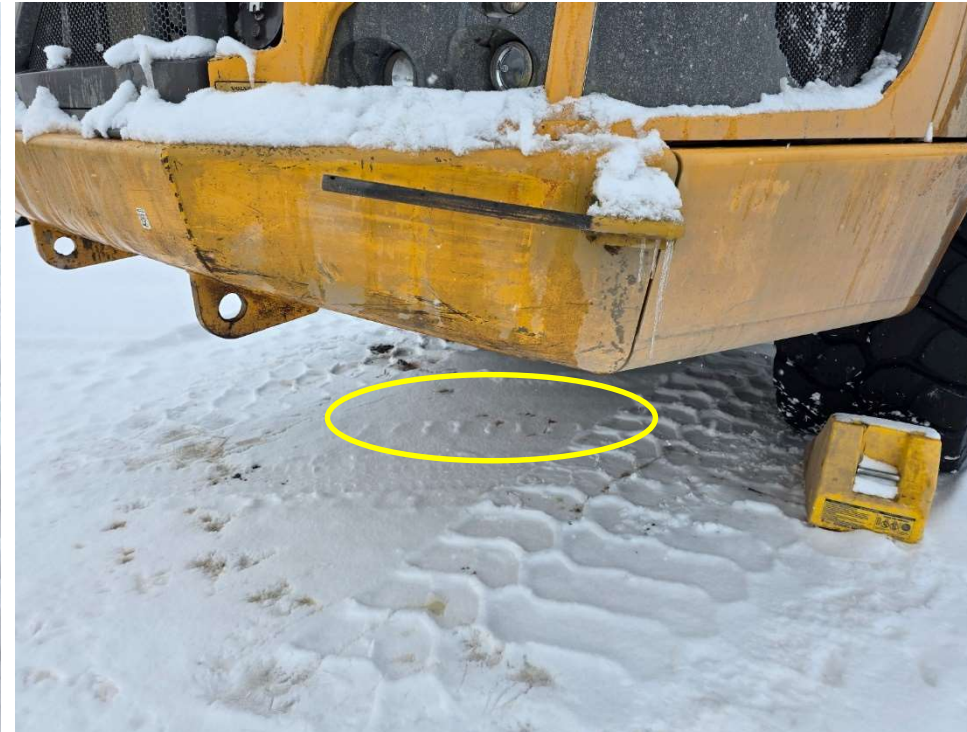
Photo 113120-5. Coolant spills observed beneath a haul truck staged at the Mobile Maintenance Yard.
