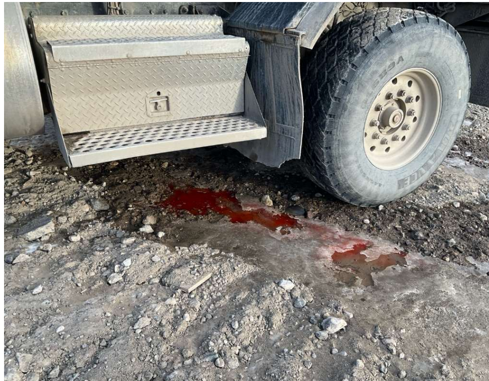
Photo 112948-4. Spill to ground observed beneath a low-bed truck staged at the 'Andrew's Hill' laydown.
