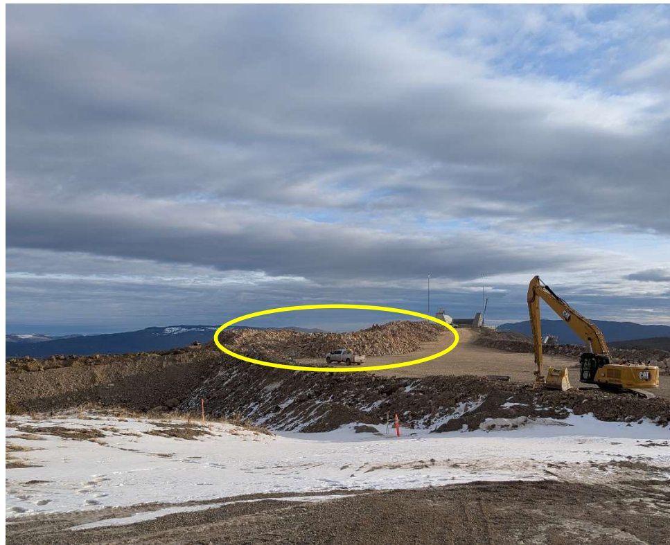
Photo 112951-2. High-grade ore stockpiled on the ROM pad adjacent to the hopper for the conveyor/crusher circuit.
