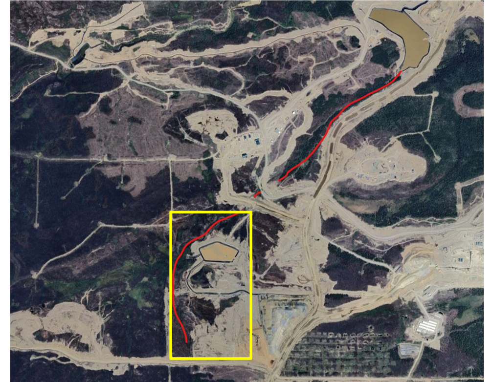
Photo 9. Approximate area where various ESC and water management measures will be installed to attempt to improve the quality of water that flows into the WMP. Approximate pathway of Mine Creek (which drains into the WMP) is included in red on drawing for reference.
