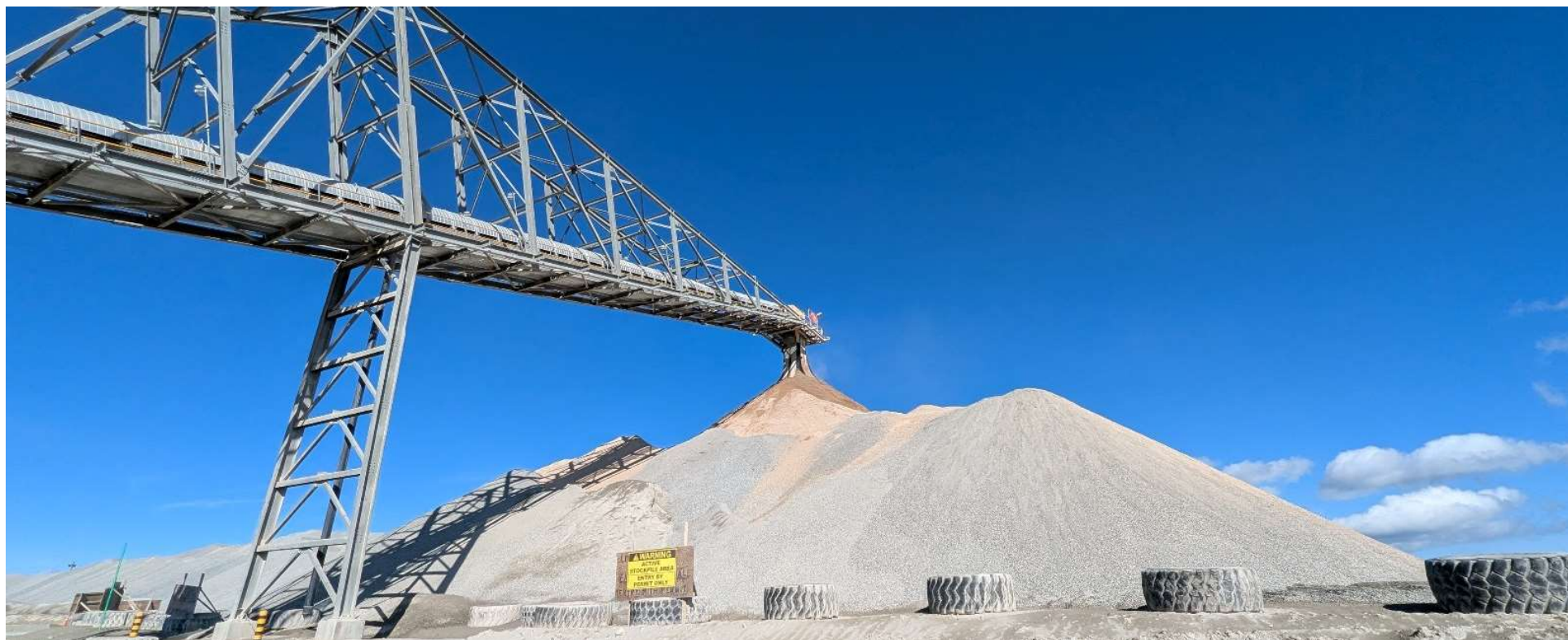
Photo 114312-1. Overview of high-grade ore stockpile at the Plant Site. BWG advised sprayers have recently been installed near the drop point from the conveyor to the pile.
