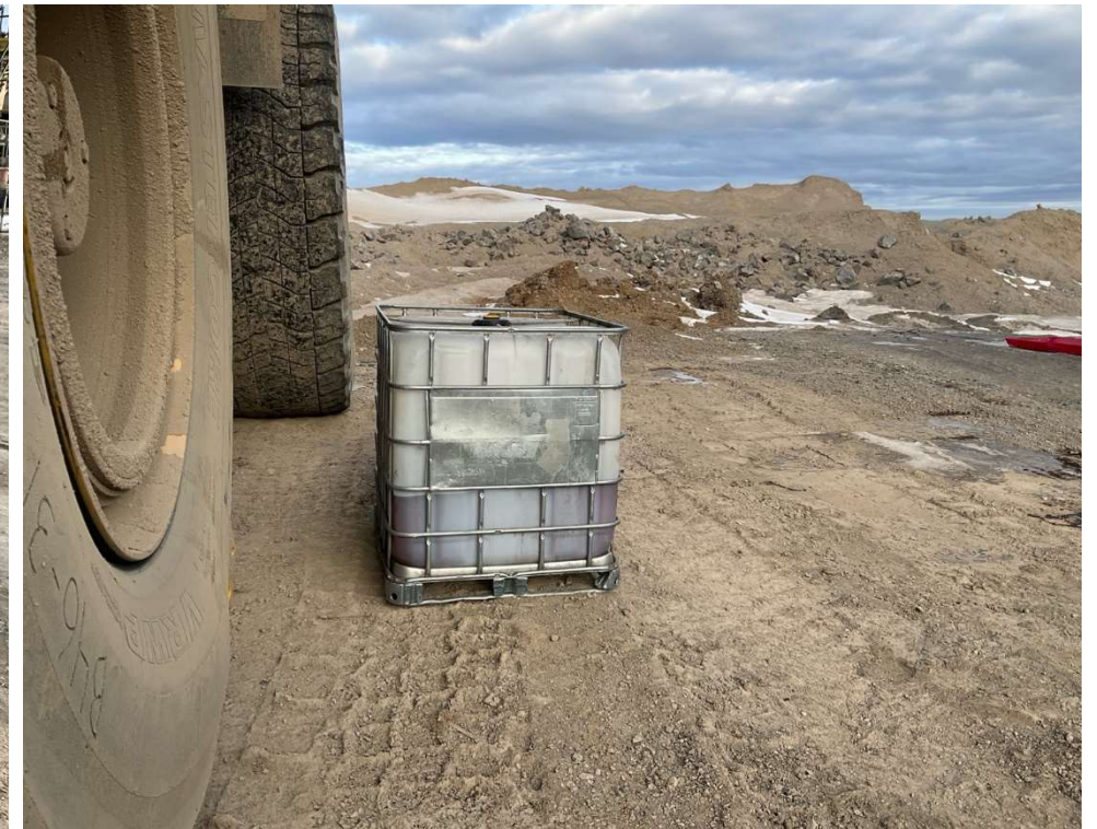
Photo 112949-1. Tote containing hydrocarbons drained from haul truck 306 at the 'Andrew's Hill' laydown. BWG confirmed tote has been removed and placed into appropriate secondary containment.
