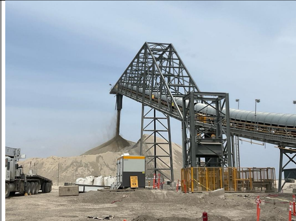
Photo 113867-4 Stockpile of high-grade ore at the drop point of the till conveyor.
